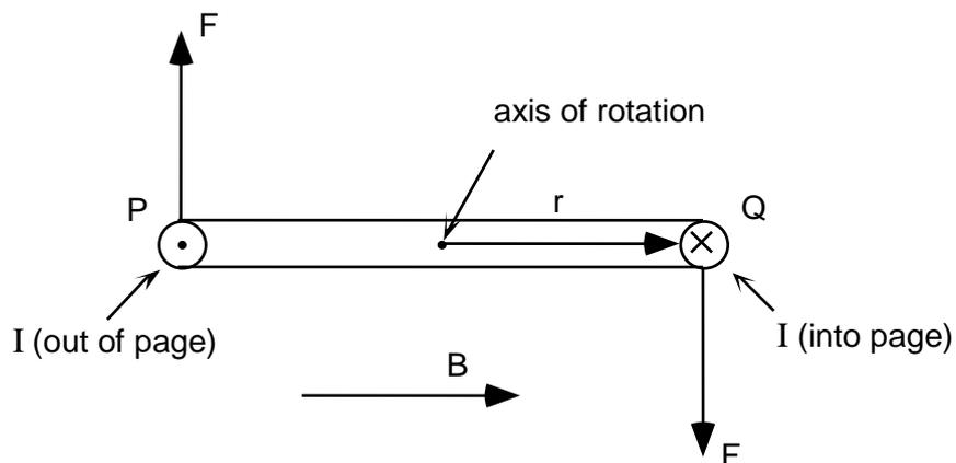
As the coil rotates,  $F$  remains constant (and is always perpendicular to the  $B$  field) but  $r$  varies (causing a change in  $\tau$ ). Torque is maximum when the plane of the coil lies parallel to the  $B$  field and reduces to zero when the plane of the coil is perpendicular to  $B$ .
