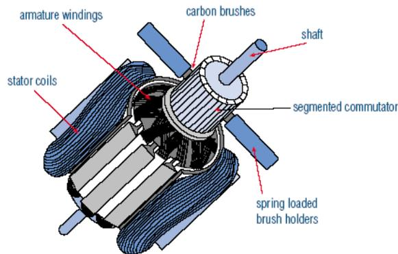
The brushes are also an important part of the electrical supply mechanism. Their function is to make electrical contact with the rotating commutator. A common material used for brushes is graphite, which is a good conductor and very slippery, hence making a low friction electrical contact.
