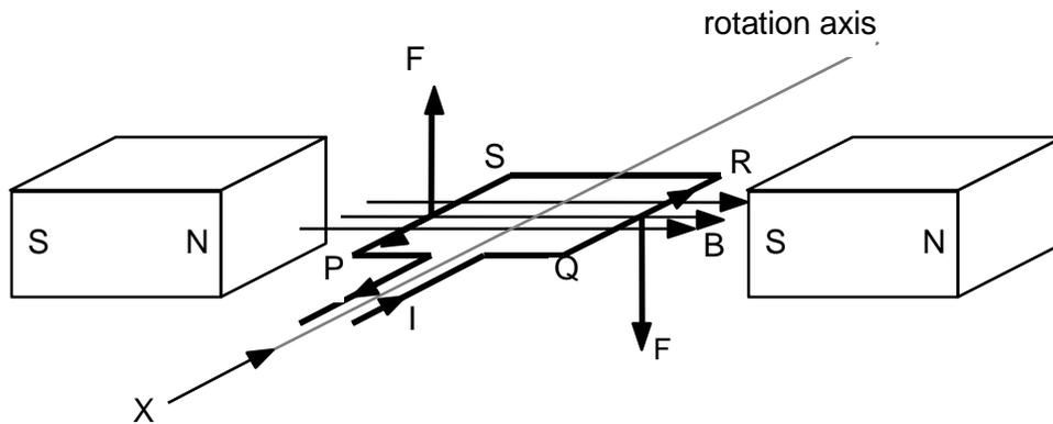
Use the Right Hand Rule to determine the direction of the forces and thus the direction of rotation. In the diagram above we can clearly see that the force on side PS is upwards, and this force, in conjunction with the downward force on side QR, causes the coil to rotate in a clockwise direction.
