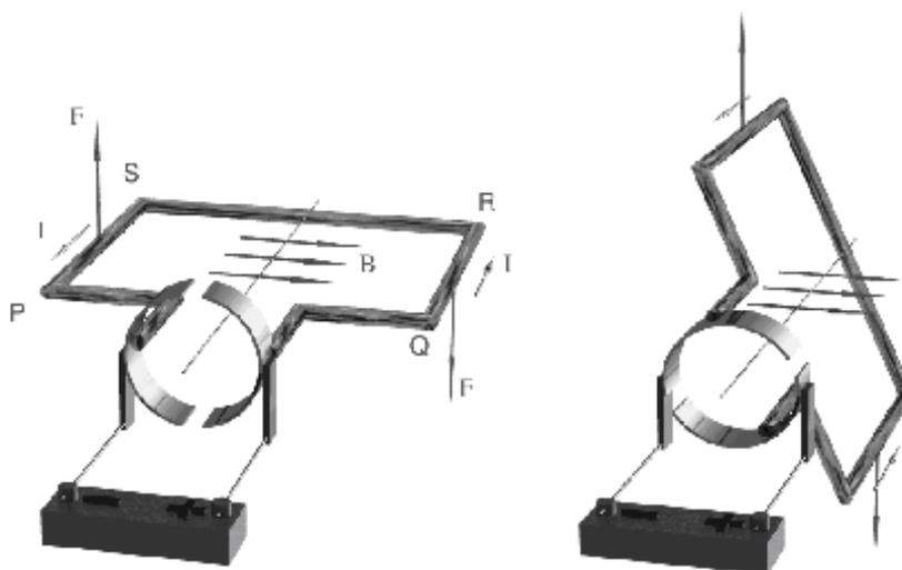
As the coil moves into the vertical position, the forces on the sides PS and QR are vertical and there is no component of the force in the direction of rotation. Therefore, at this position the applied forces on PS and QR does not contribute to rotation.
